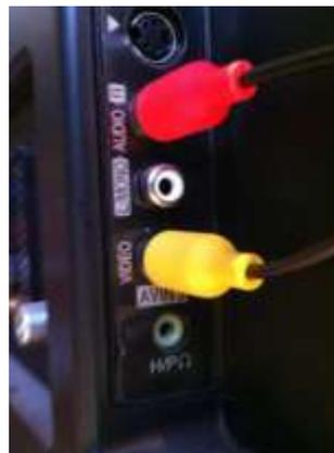
6. If you have not already done so, make sure that the input on your TV or Display has been switched to it's composite input channel (i.e. the channel that relates to the socket where you have connected the yellow video cable from your Hero 3 camera)
