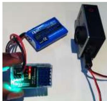
Output channel from the Voltage regulator connected to the power connector of the Camera's Video out cable (after ensuring that the Voltage regulator jumper connector has been set for 5.2volts)
