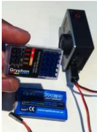
7.4v 2 Cell Lipo Battery connected to one of the 2 input sockets
