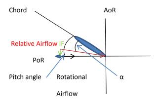
So now we have our blade being acted upon by the relative airflow at a given angle of  $\alpha$ . The blade then produces Lift at 90 deg to Relative Airflow and drag 90 deg to Lift. We then combine the two to give us Total Reaction.
