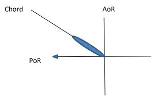
We can now draw on the Rotational Airflow and the IF. Rotational airflow acts along the PoR and IF along AoR. IF is fairly small and Rotational Airflow large in comparison.
