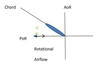
From these we can deduce the Relative Airflow. This is the airflow the blade sees. We can then take two angles. The first is the pitch angle of the blade and the second is Alpha ( $\alpha$ ) or AoA.
