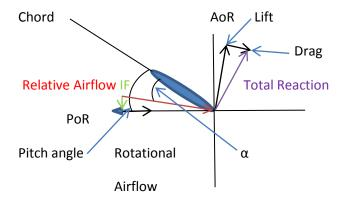
Nearly there. Ok, we can separate the Total Reaction into its constituent vectors on the X and Y axis and these give us the Rotor Drag and Total Rotor Thrust(TRT). These two forces are countered by Thrust (or in a helicopter Torque(Tq)) and Weight and when these are balanced we are in a steady state. For the purpose of this example we said we were in a hover, so if nothing changes we will remain hovering.
