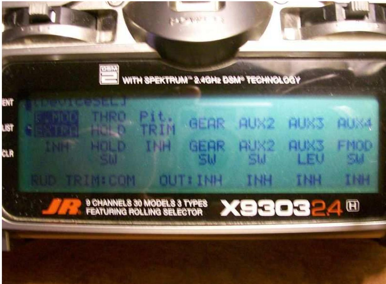
Step 1, picture above. Because switches will now be used for mix they must be inhibited! Enter system mode by powering on TX with ent. button pressed in then select device select and set screen as above.
