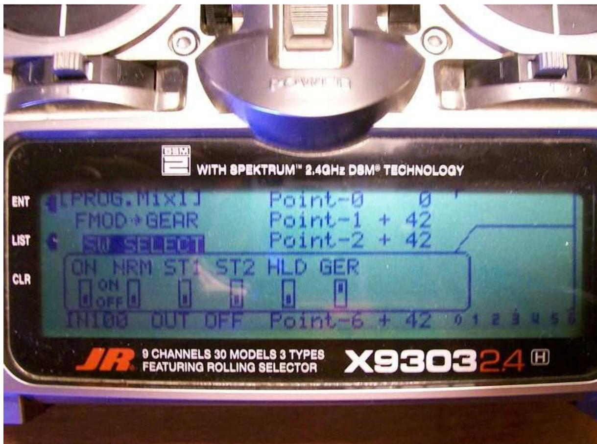
Step 3, picture above. Still in programmable mix 1 select switch select and move the little box to the on position in the gear window ONLY. You will now notice that when the gear switch is up the mix is off and when the gear switch is down the mix is turned on which will be heading hold. The next step will regain the use of the gear switch in the up or 0 position for rate mode!
