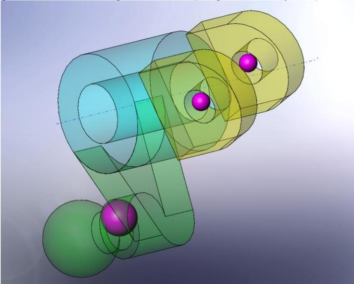
**6.** Add the tail blade. The point masses of the blade are in line with the pitch arm and ball. That means whatever torque they generate will add to the torque generated by the pitch arm and ball increasing the overall tennis racquet torque.
