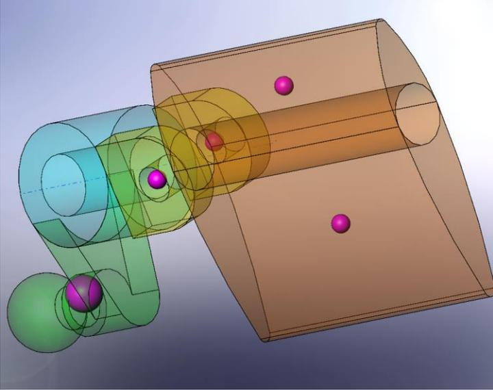
**7.** Add the blade bolt and nut. The point masses of the blade bolt and nut added are at 90 degrees to the pitch arm, ball and blade. That means whatever torque they generate will work against the torque generated by the pitch arm, ball and blade reducing the overall tennis racquet torque. This shows why adding mass to the blade bolt and nut decreases tennis racquet effect.
