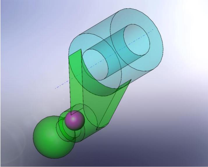
**5.** Add the blade grip ears to the hub. The point masses of the blade grip ears added are at 90 degrees to the pitch arm and ball. That means whatever torque they generate will work against the torque generated by the pitch arm and ball reducing the overall tennis racquet torque.
